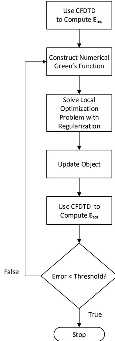
Fig. 2: Inversion Flow Chart with CFDTD Forward Solver and Integrated Numerical Green's Function.
