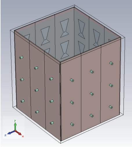
Fig. 1: CAD Drawing of Prototype Imaging Cavity
