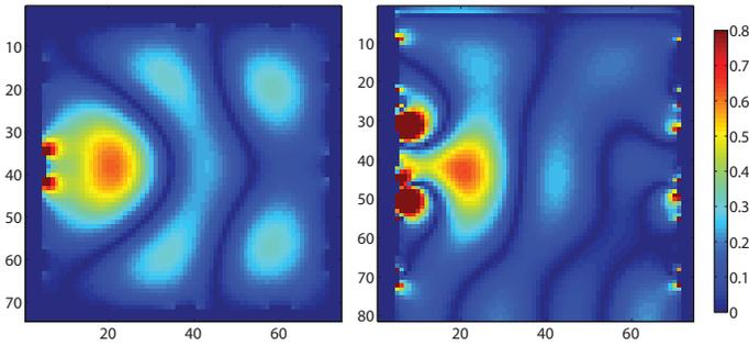
Fig. 4:  $|Re(E_z)|$  Due to Single Transmitting Antenna at Resonance. (Left) Top View of Horizontal Cut (xy) Through Cavity, (Right) Side View of Vertical Cut (xz) Through Cavity
