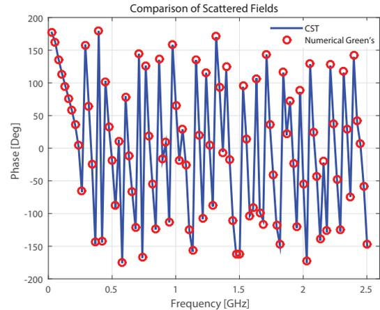
Fig. 5: Scattered fields comparison between FDTD solver and numerical Green's function estimation. Magnitudes agree within a mean absolute difference of 0.2 dB. Phases agree within a mean absolute difference of 2 degrees.
