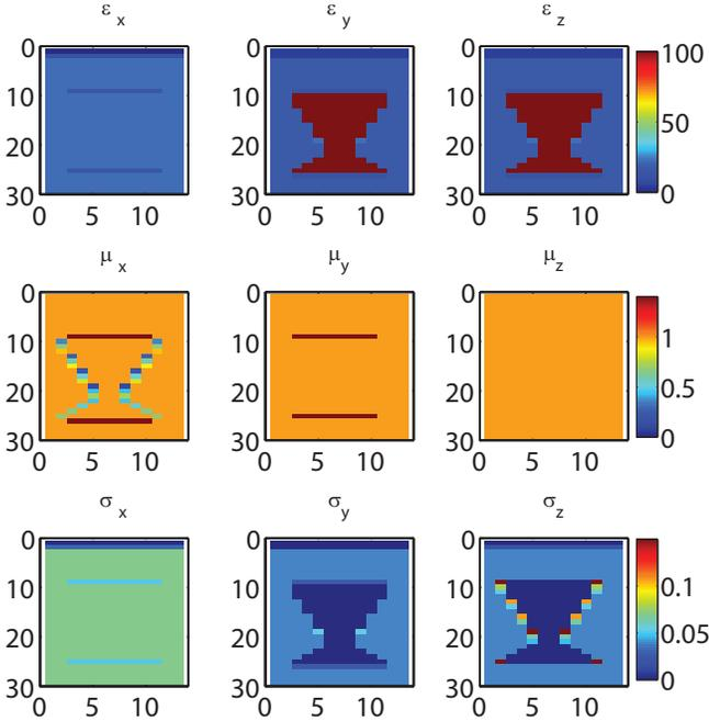
Fig. 3: Effective Materials (Row 1:  $\epsilon$ , Row 2:  $\mu$ , Row 3:  $\sigma$ ) Used to Model Antennas in Imaging Cavity with CFDTD
